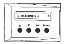
The above diagram shows the four control buttons and LCD display on the DTC. The DTC has 2 main menu options, "**READINGS**" and "**ADJUSTMENTS**".
