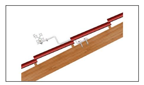
If the pantile is profiled, there might be a need to locate the roof hook to the joist using the mounting plate as a connector. Here is an example:
