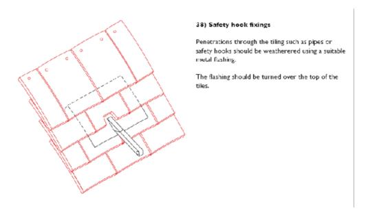
For slates, the tiles will need to be drilled. The internal rafters can be located by feeding an aluminium strip out from the loft between the felt sarking layers and then abutting the aluminium strip against the roofing rafter. The external exposed end of the aluminium will indicate the location of the internal rafter. Alternatively, use noggins between the rafters to firmly locate the aluminium strips.
