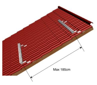
removed to locate the hooks can be replaced. The top and bottom mounting bars can then be bolted to the roof hooks.
