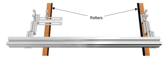
This example is based on a roof with a timber sarking. If no timber sarking is available, the nuts, bolts and spring washers as provided can be used to bolt the roof hook to the mounting plate. Another alternative is to place a noggin between the rafters to strengthen the mounting structure and screw the roof hook to the noggin.
