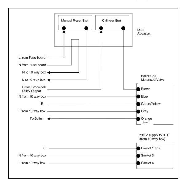
Alternatively, two manual reset thermostats can be employed on the heating system. One thermostat, located to respond to the boiler coil, is wired conventionally as per manufacturer's instructions to the boiler heating controls and the solar manual reset thermostat,
