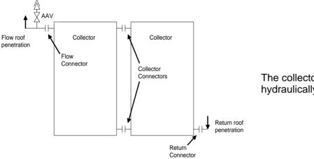
The collectors should be hydraulically piped as follows:
